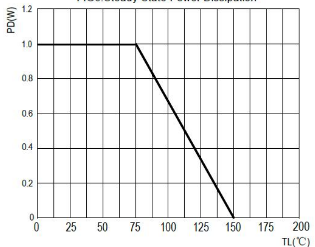
FIG6: Steady State Power Dissipation
